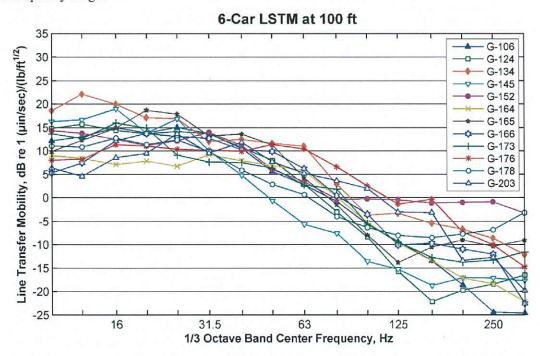
Figure 2: Cross-site Comparison of LSTM Values (6-Car trains at 100 Foot Diagonal Distance)
