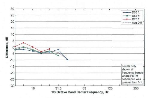
Figure 34: LSTM Difference (Indoor - Outdoor) for Room 123
