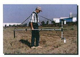
Geometrics G858 Cesium Magnetic Gradiometer
