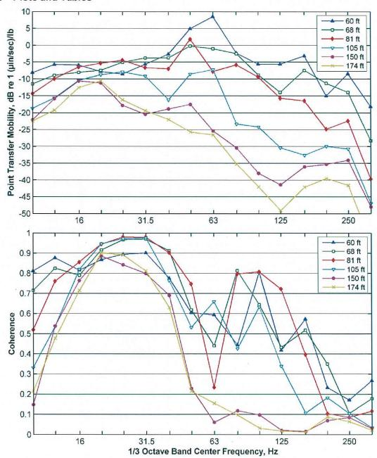
Figure 37: G-166. Measured PSTM at Depth of 55 ft
