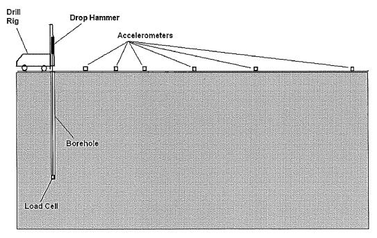
Figure 3: Borehole Test Configuration
