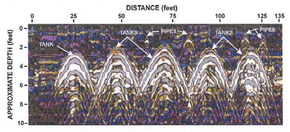
GPR Survey to Locate Underground Storage Tanks
